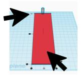
Click on the cylinder. Use the down arrow key on the keyboard to position the hole vertically. (Do not use the right or left keys or you will need to re-align it.) Click the down arrow key 7 times to move the hole down 7 mm.
