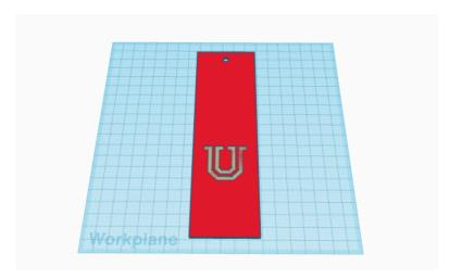
In the pop-up window change the largest dimension to 100 mm. Once your file has imported, adjust the dimensions as necessary. Don't forget to adjust the height.
